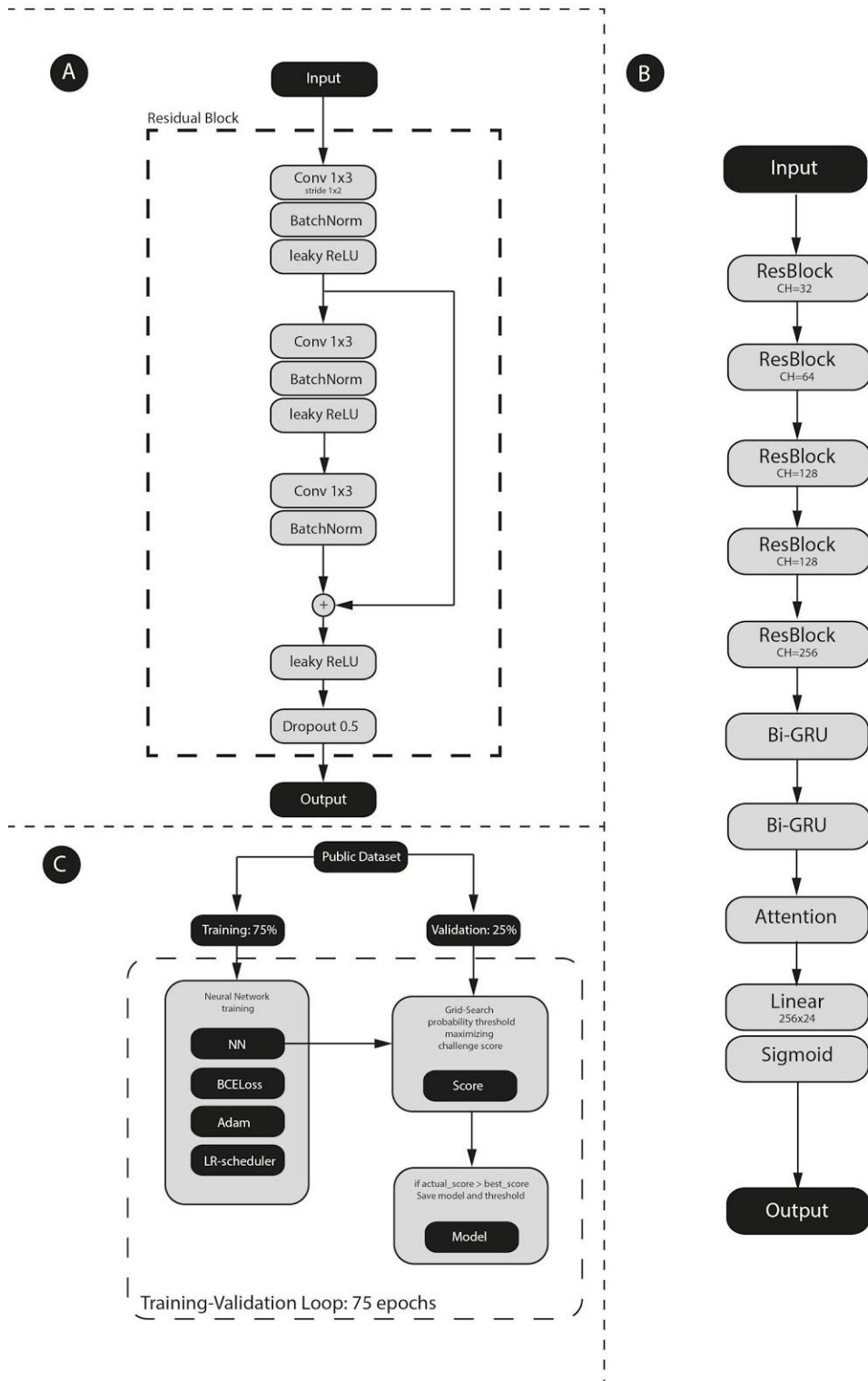
Figure 1. The picture depicts A) residual block architecture, B) full model architecture, and C) training and validation pipeline with grid-search threshold optimization
