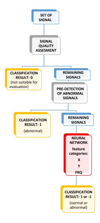
Fig.1 Flow chart of PCG classification algorithm.
