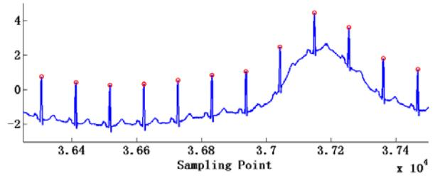
Figure 2. Detected QRS complex by the Tompkins difference algorithm.
