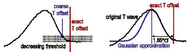
Figure 2. Exact T offset detection. Two independent methods for exact wave boundary calculation were used and averaged: Left: decreasing thresholds for the range curve. Right: Gaussian approximation to the descending T wave.
